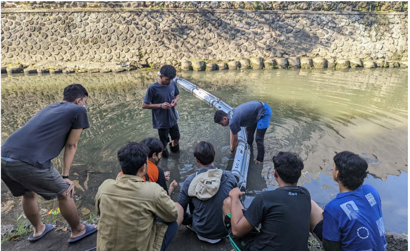
Image: Evaluating the effectiveness of a trash boom on a river in Indonesia as part of the PISCES GCRF Project. © Dr Max Kelly.
